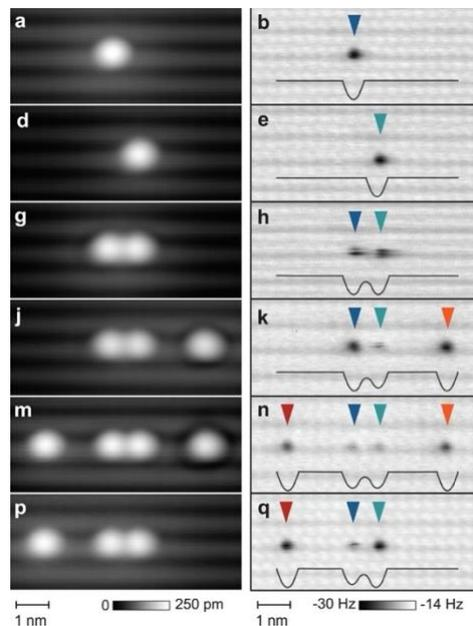
has responded to this field change by moving to the right. Measurement and *ab initio* calculation show that the bit energy, that is the energy required to change binary state is roughly  $10^{-20}$  Joule. Taken together, these data show our unique, unprecedented ability to represent and control information using very little energy.
